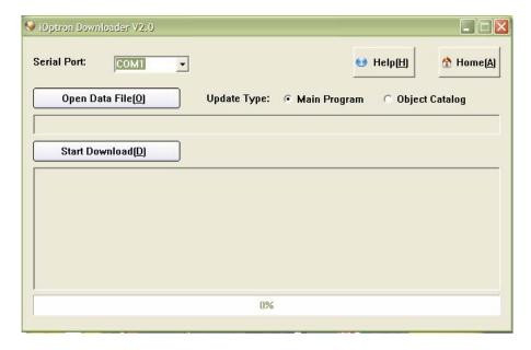
On the interface, select appropriate port using pull-down menu (in this case, COM4):
