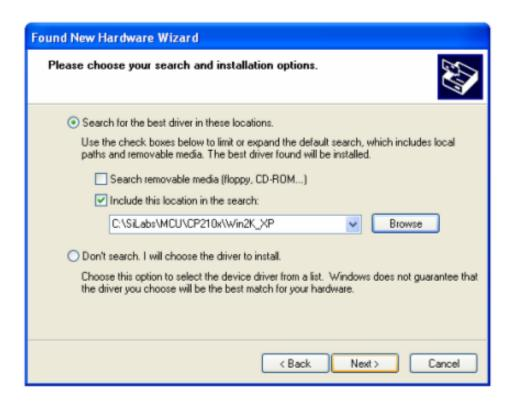
Click "Next". The computer will starting to install the driver for the USB2COM. When the installation is done, click "Finish".
